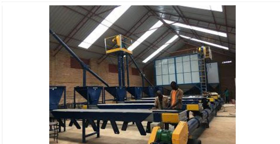
6 new conveyor belts for sorting green coffee. Automated movement to the "mixing silo" at the back.
